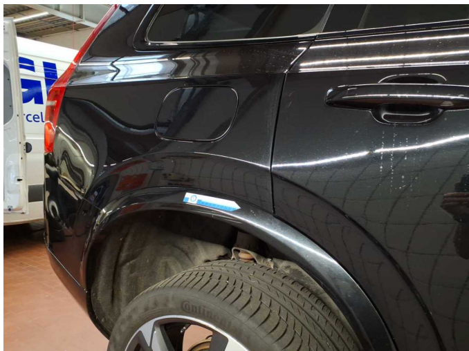
Damage 7: Side panel - rear right side: Wheel well extension - Scratch(es) - Smart repair
