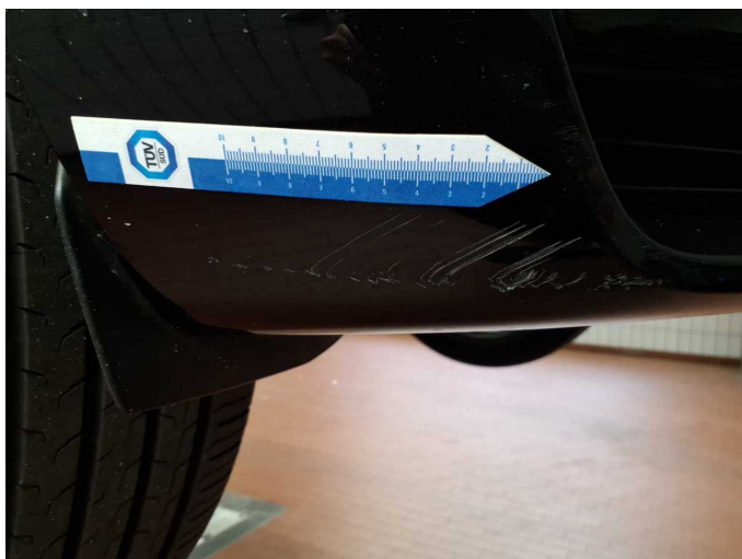
Damage 8: Front bumper: Spoiler - Scratched - Smart repair
