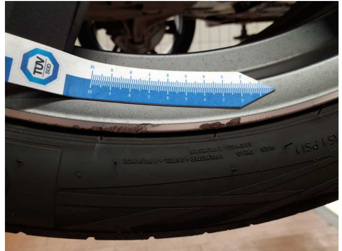
Damage 15: Wheel / tyres: Alloy rim - front left side - Scratched - Loss in value
