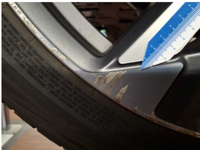
Damage 16: Wheel / tyres: Alloy rim - front right side - Scratched - Loss in value
