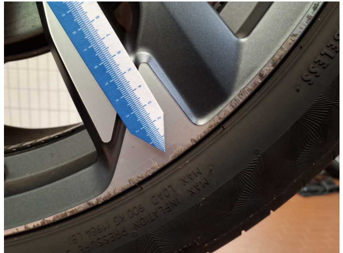
Damage 14: Wheel / tyres: Alloy rim - rear left side - Scratched - Loss in value
