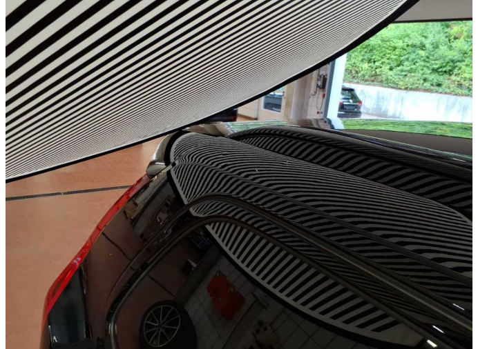
Damage 17: Body: Body - Damage by hail - repair according to calculation
