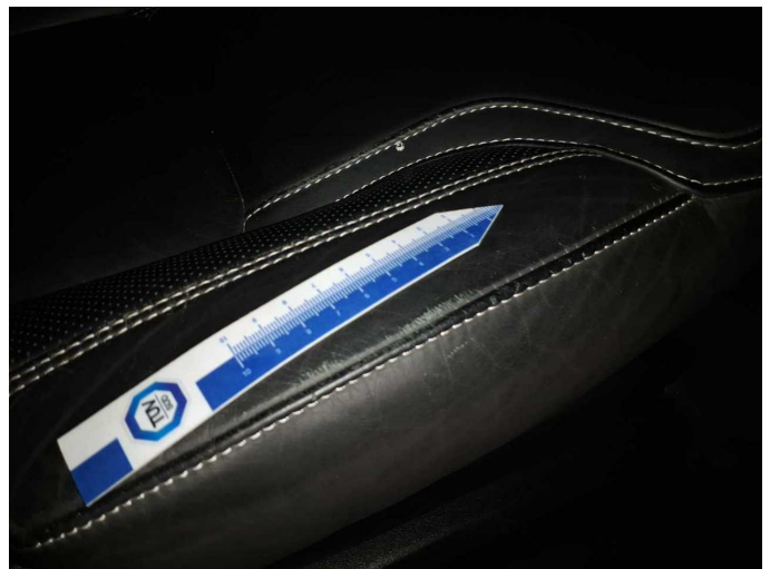
Damage 3: Seat - rear: Seat cover - 3 seater bench - Scratch(es) - Smart repair
