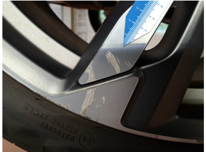
Damage 13: Wheel / tyres: Alloy rim - rear right side - Scratched - Loss in value
