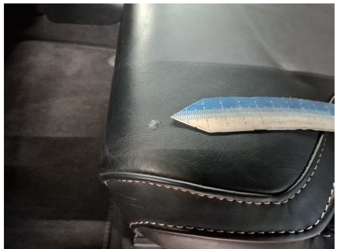
Damage 4: Seat - rear: Upholstery - Scratch(es) - Smart repair
