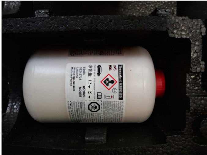
Damage 1: Equipment: Tirefit filler - Due - Replace
