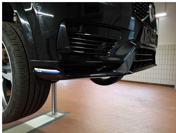
Damage 8: Front bumper: Spoiler - Scratched - Smart repair
