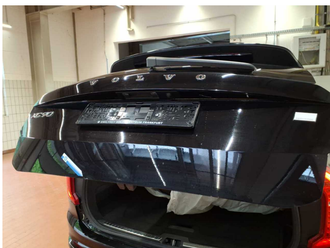
Damage 12: Boot lid / rear door: Boot lid - Dent / paintcoat damage - Smart repair
