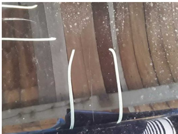
Damage #9: Boot lid / rear door: Boot lid - Scratched - Paint
