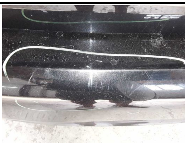
Damage #8: Rear bumper: Rear bumper - Scratched - Paint
