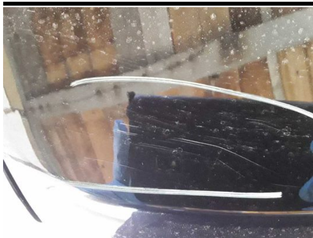
Damage #9: Boot lid / rear door: Boot lid - Scratched - Paint
