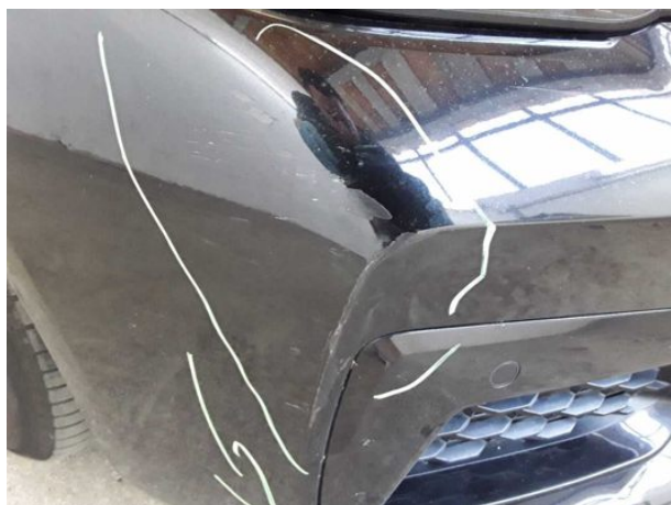
Damage #10: Front bumper: Front bumper - Deformed - Repair a... paint
