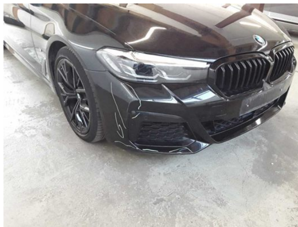
Damage #10: Front bumper: Front bumper - Deformed - Rep... and paint
