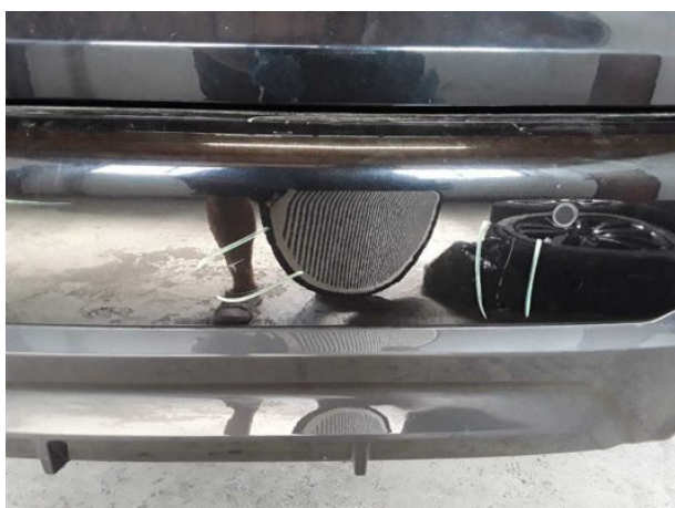
Damage #8: Rear bumper: Rear bumper - Scratched - Paint
