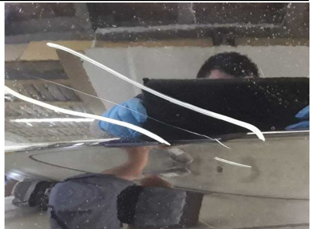
Damage #6: Mudguard - left side: Mudguard - left side - Scratched - Paint
