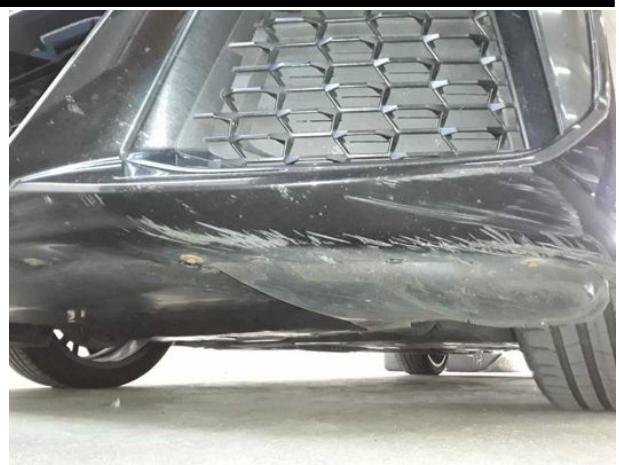
Damage #10: Front bumper: Front bumper - Deformed - Repair and paint
