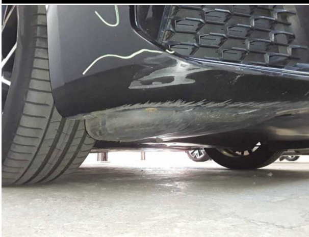
Damage #10: Front bumper: Front bumper - Deformed - Repair and paint
