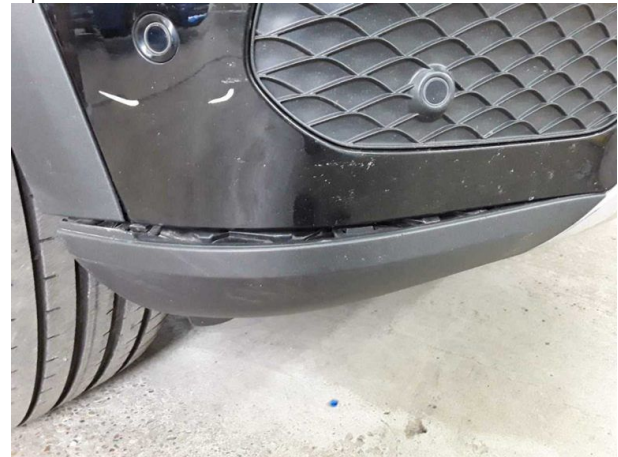
Damage #6: Front bumper: Spoiler - Loose - Diagnosed and repair if necessary
