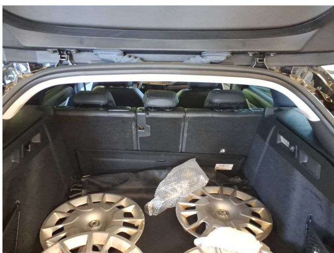
Missing part 1: Interior: Rear shelf - Missing - Replace
