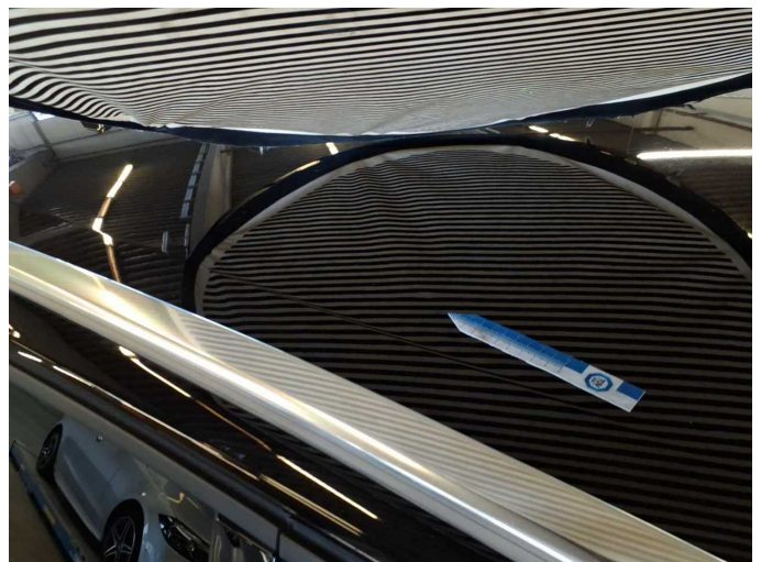
Damage 1: Roof: Roof - dent(s) - Smooth repair work
