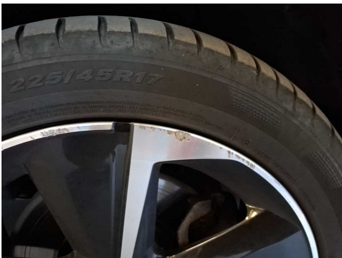
Damage 8: Wheel / tyres: Alloy rim - front right side (Materialabtrag) - Scratched - Replace
