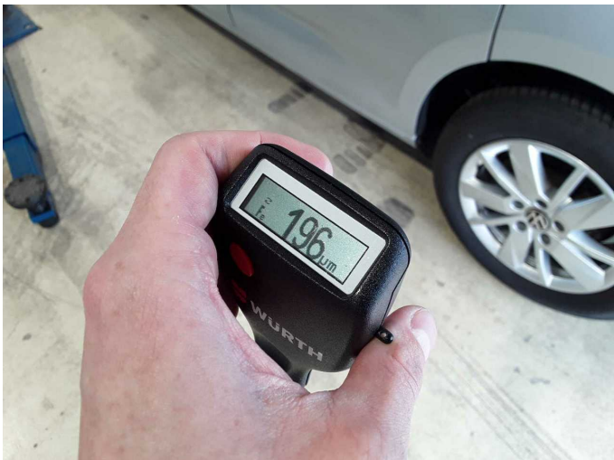
Repainting 1: Door - rear left side
