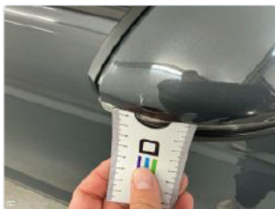
11 - Outside rear-view mirror housing R - Scratch(es)
