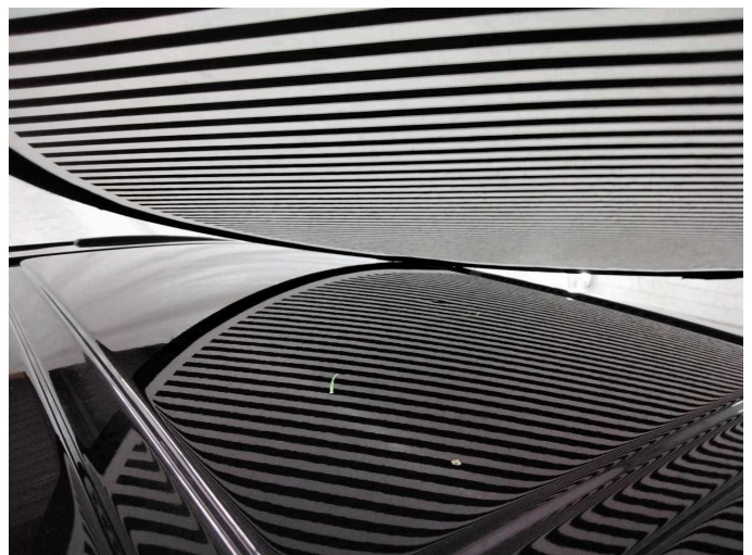
Damage 3: Roof: Roof - dent(s) - Smooth repair work
