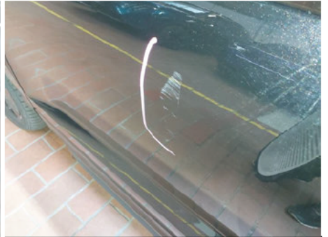
Tür / Vorne Links / Kratzer
