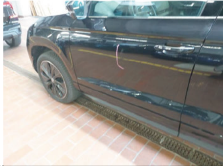
Tür / Vorne Links / Kratzer
