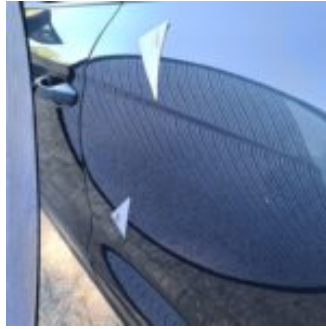
Damage Type Small dent(s)
