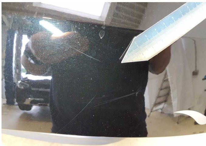
Damage 5: Boot lid / rear door: Boot lid - Scratch(es) - Paint
