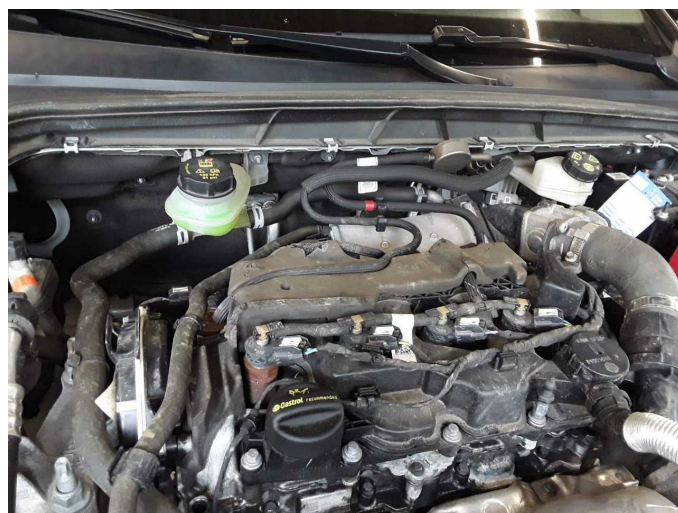
Damage 3: Engine: Engine cover - Damaged - Replace
