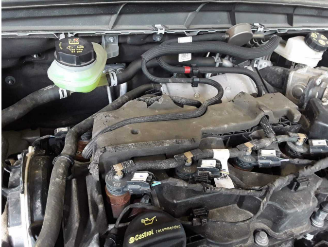
Damage 3: Engine: Engine cover - Damaged - Replace
