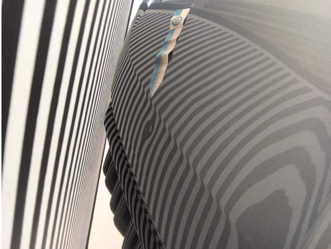
Damage 3: Bonnet: Bonnet - dent(s) - Smooth repair work
