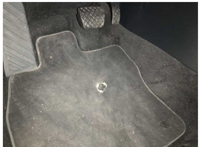
Damage 1: Trim / covers: Floor mats - Damaged - Replace
