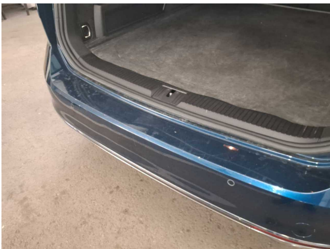
Damage 5: Rear bumper: Rear bumper (Ladekante) - Scratched - Paint
