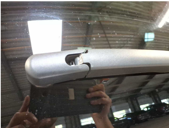
Damage 3: Screen cleaning: Wiper arm - rear - Broken / torn - Replace
