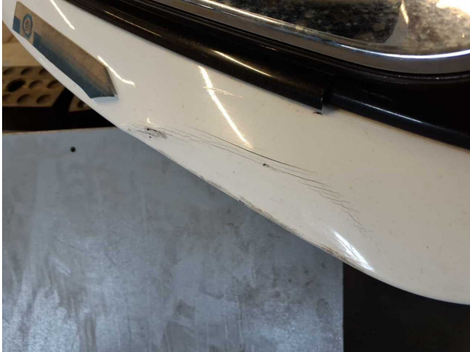
Damage 12: Front bumper: Front bumper - Damaged - Replace
