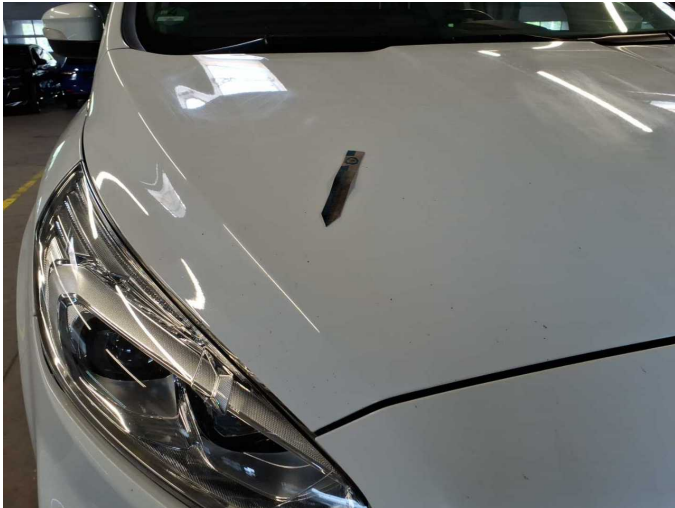
Damage 11: Bonnet: Bonnet (Steinschlag) - Scratched - Paint
