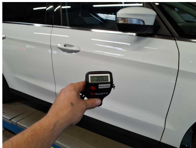
Repainting 2: Door - front right side
