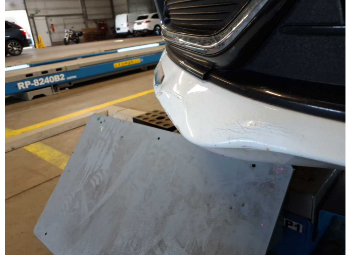
Damage 12: Front bumper: Front bumper - Damaged - Replace
