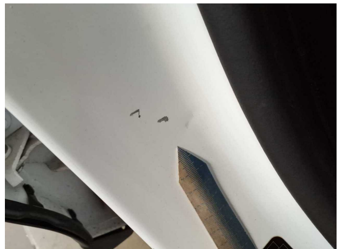
Damage 9: Sill - right side: Sill - Dent / paintcoat damage - Smart repair
