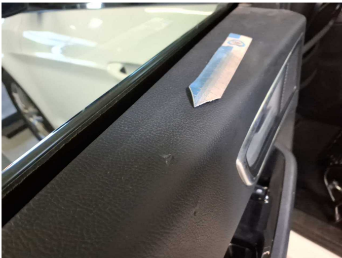
Damage 10: Trim / covers: Door trim - rear left side - Broken / torn - Smart repair
