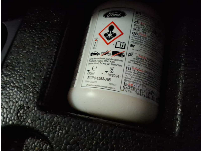
Damage 2: Equipment: Tirefit filler - Expired - Replace
