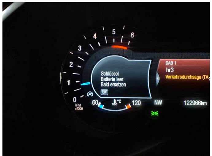
Damage 1: Equipment: Vehicle key (Batterie) - Empty - Replace
