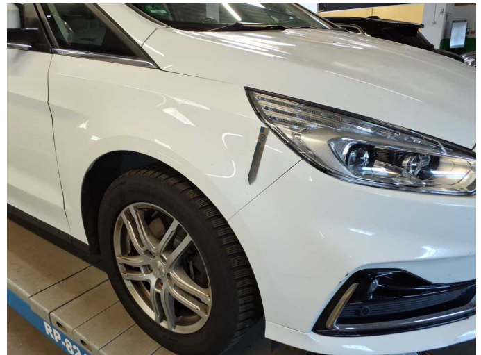
Damage 6: Mudguard - right side: Mudguard - right side - Stone chips - Smart repair
