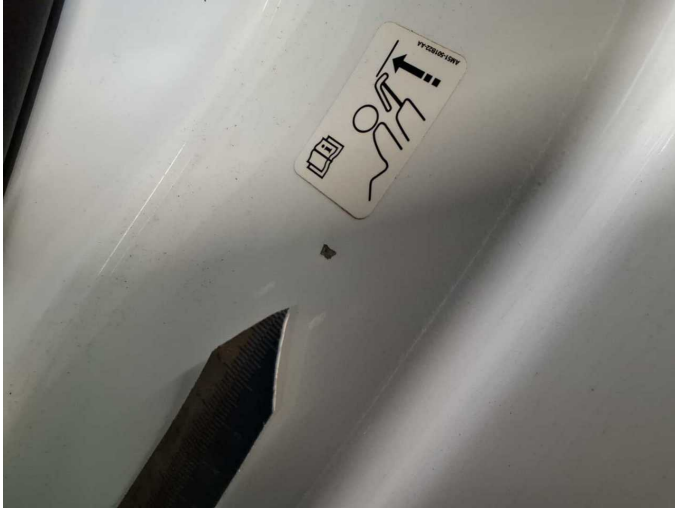
Wear and tear 3: Side panel - rear left side: Sill - Scratch(es) - Cover / polish
