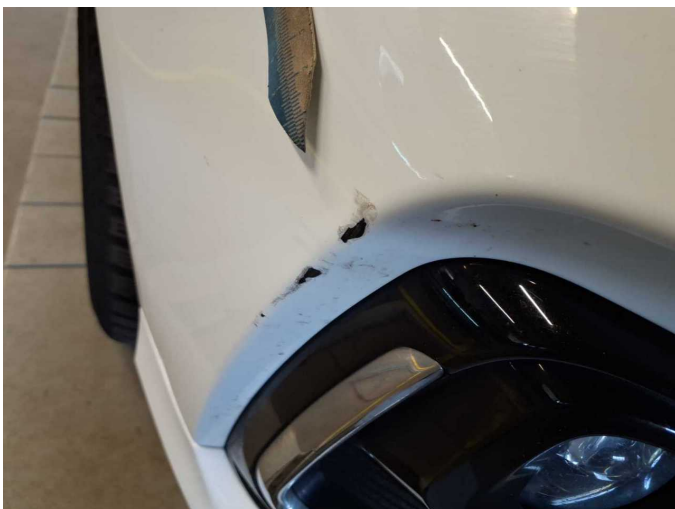
Damage 12: Front bumper: Front bumper - Damaged - Replace
