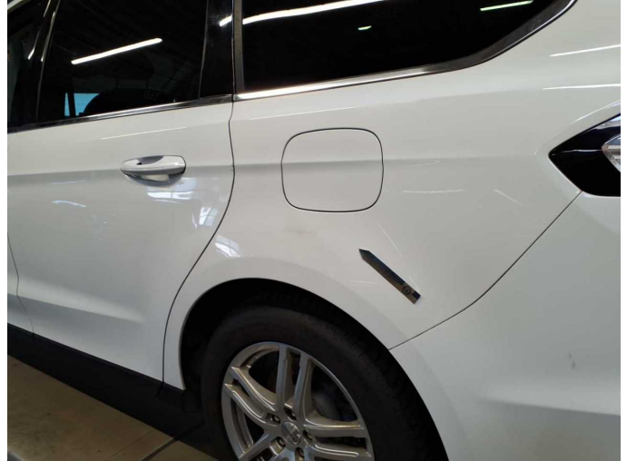
Wear and tear 4: Side panel - rear left side: Side panel (polieren) - Scratched
