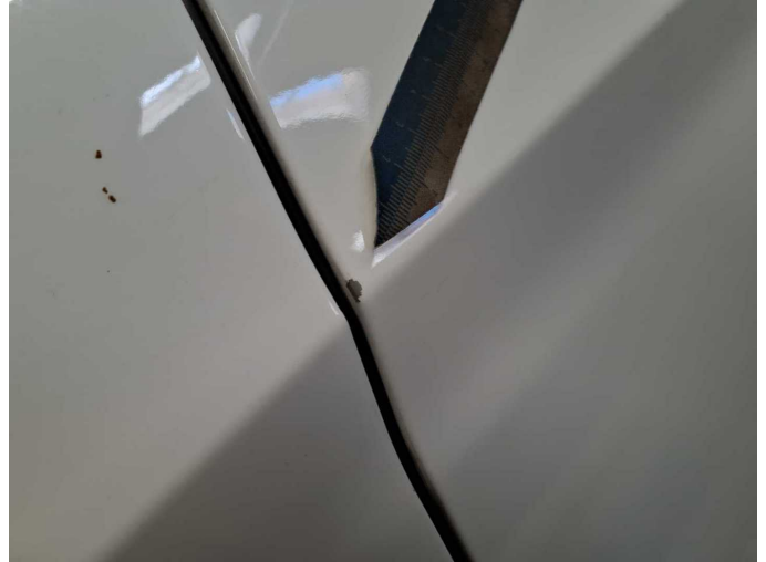
Damage 7: Door - rear left side: Door - Scratch(es) - Smart repair
