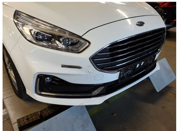
Damage 12: Front bumper: Front bumper - Damaged - Replace
