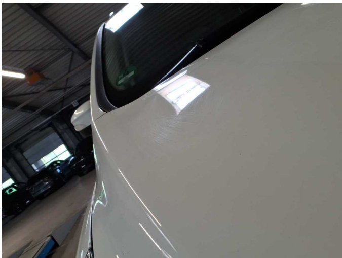
Damage 11: Bonnet: Bonnet (Steinschlag) - Scratched - Paint
