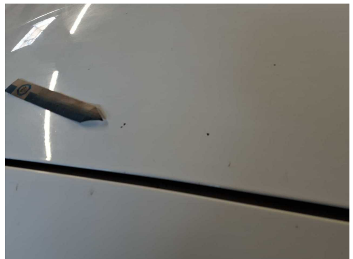
Damage 11: Bonnet: Bonnet (Steinschlag) - Scratched - Paint
