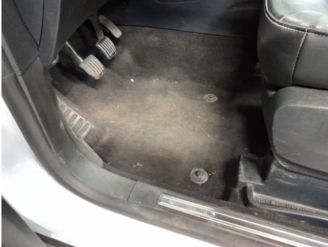
Damage 5: Trim / covers: Floor covering - front left side - Burn hole (cigarettes) - Smart repair
