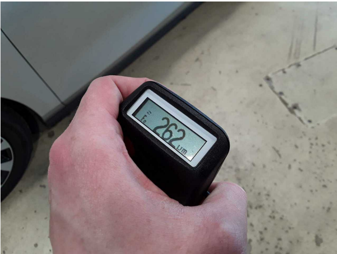
Repainting 1: Door - front left side
