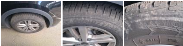
Tyre RR, Out of tolerance, Replace
