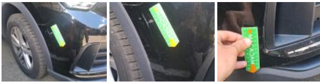
Bumper moulding F, Deformed / Strained, Replace
