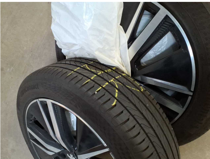
Damage 7: 2nd wheel set: 2 alloy rims (Materialabtrag) - Scratched - Replace
