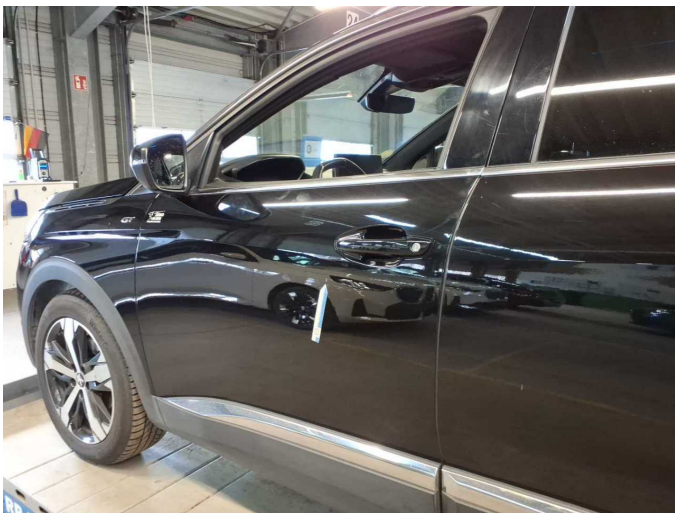
Damage 5: Door - front left side: Door - Dent / paintcoat damage - Repair and paint
