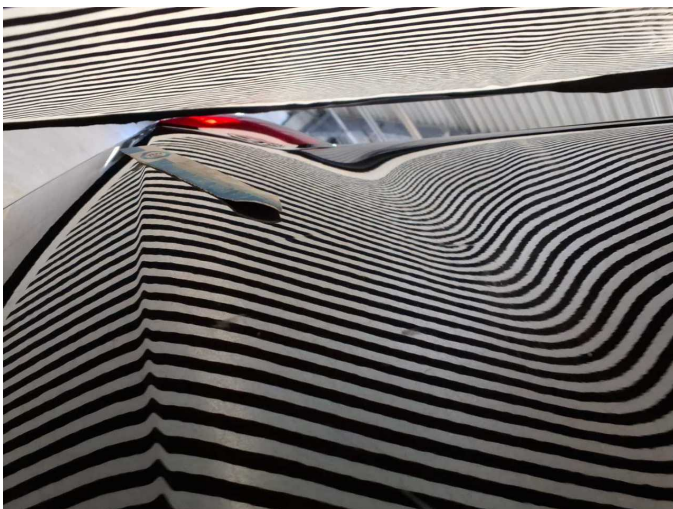
Damage 6: Side panel - rear right side: Side panel - Dent / paintcoat damage - Smart repair
