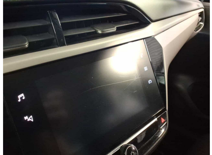
Damage 8: Multimedia system: Entertainment (Display) - Scratched - Loss in value
