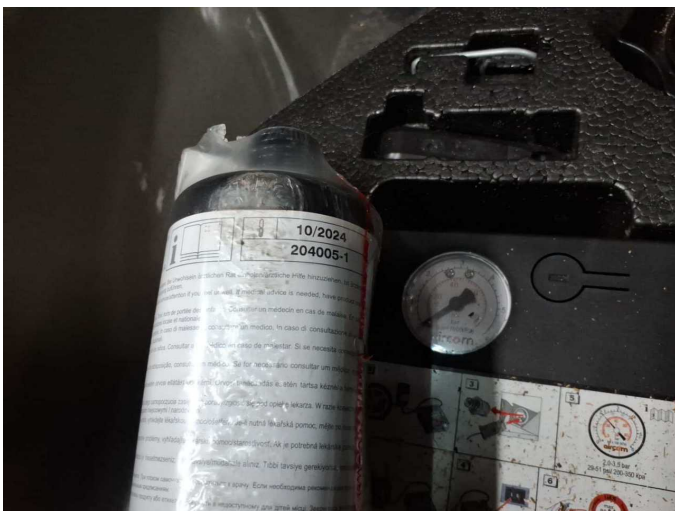
Damage 1: Equipment: Tirefit filler - Expired - Replace
