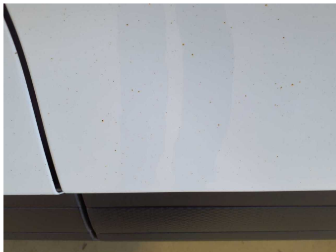
Damage 8: Body: Body (Flugrost) - Stone chips - Conditioning
