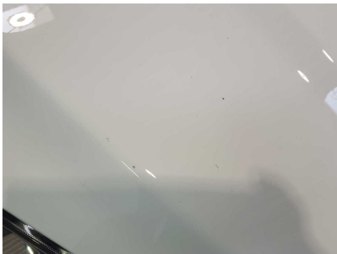
Damage 11: Bonnet: Bonnet - Stone chips - Paint
