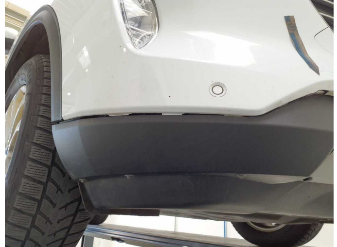
Damage 14: Front bumper: Front bumper (Inklusive anbauteile) - Broken / torn - Replace
