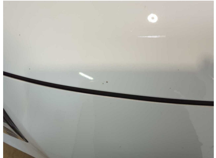
Damage 11: Bonnet: Bonnet - Stone chips - Paint
