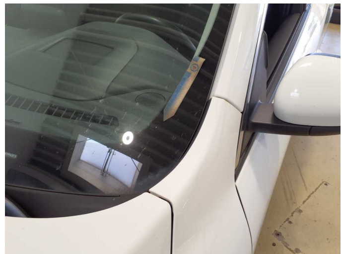
Damage 12: Vehicle glazing: Windscreen - Stone chips - Replace
