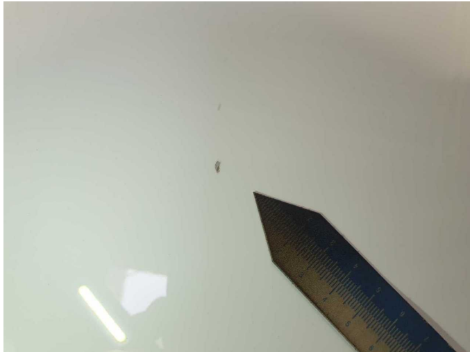
Damage 11: Bonnet: Bonnet - Stone chips - Paint
