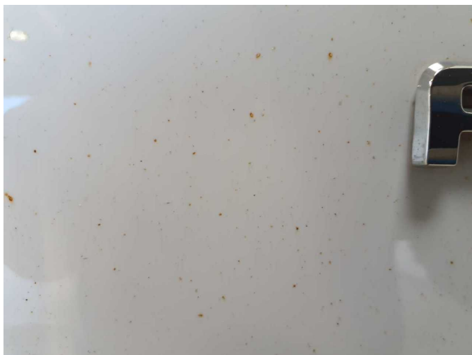
Damage 8: Body: Body (Flugrost) - Stone chips - Conditioning
