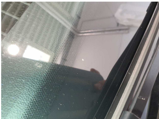
Damage 12: Vehicle glazing: Windscreen - Stone chips - Replace
