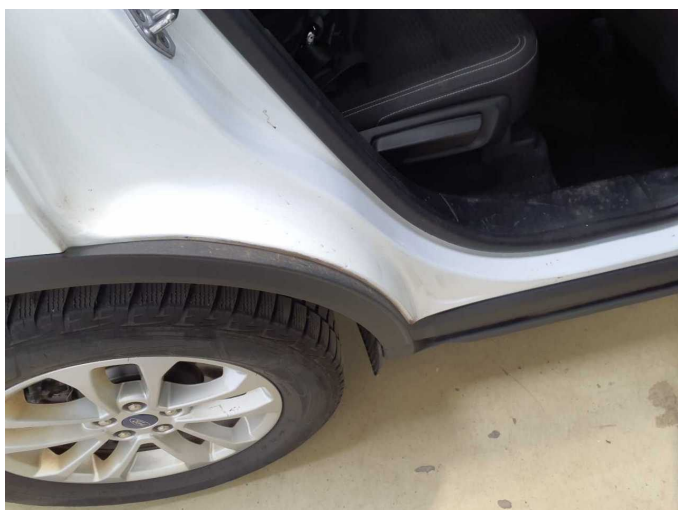
Damage 6: Side panel - rear right side: Sill - dent(s) - Smart repair
