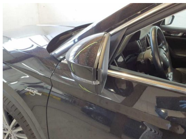
Damage #11: Wing mirror - left side: Mirror housing (+ Blinker...) Damaged - Replace
