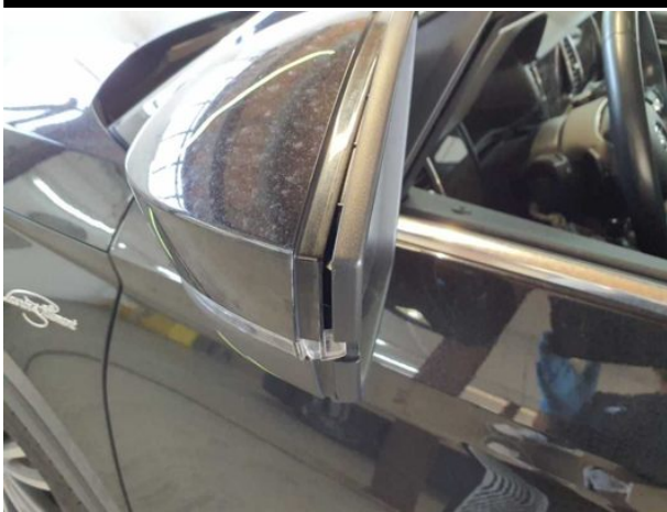
Damage #11: Wing mirror - left side: Mirror housing (+ Blinker) - Damaged - Replace
