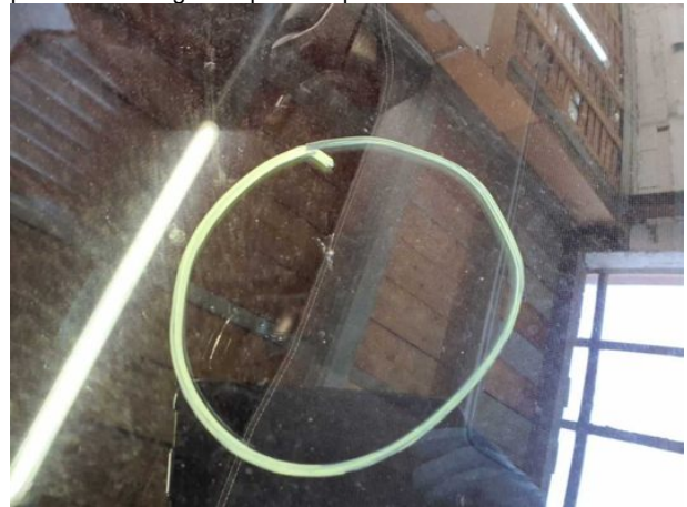
Damage #15: Vehicle glazing: Windscreen with rain sensor (... Rissbildung) - Stone chips - Replace
