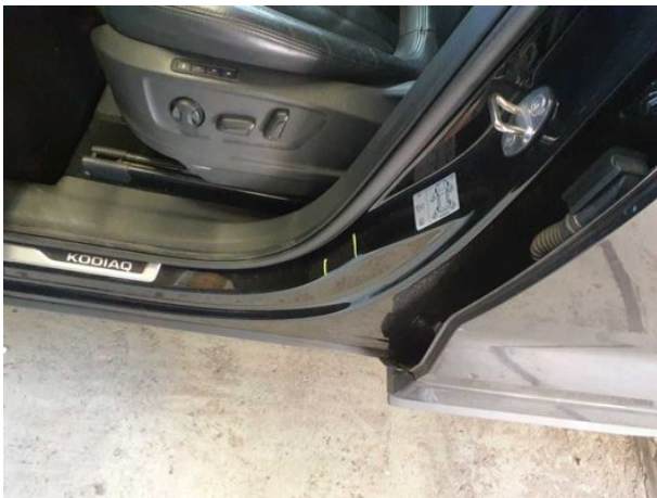
Damage #9: Sill - left side: Sill - dent(s) - Smart repair
