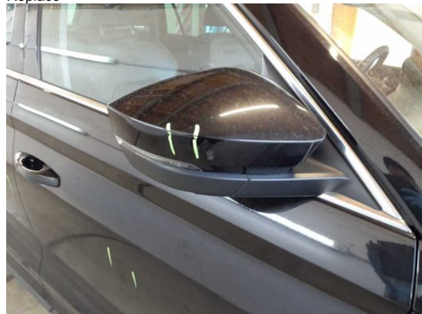
Damage #7: Wing mirror - right side: Cap - Scratched - Smart repair
