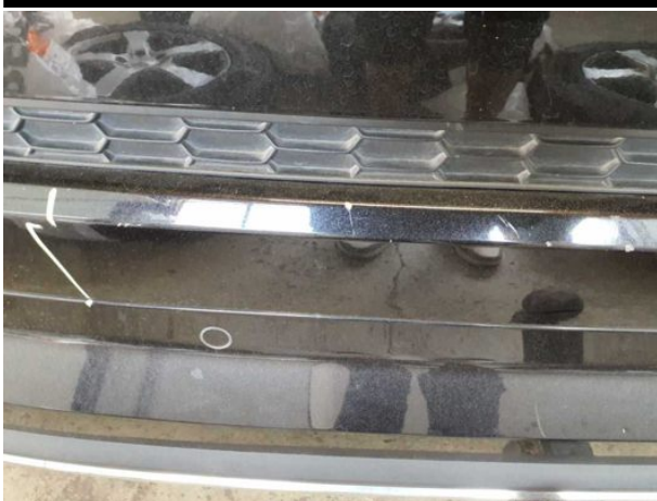
Damage #8: Rear bumper: Rear bumper - Scratched - Smart repair
