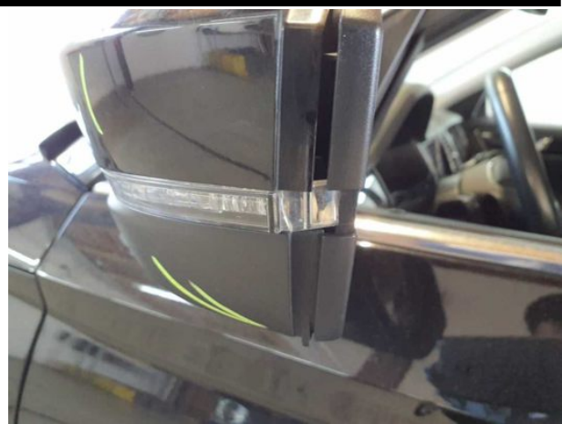
Damage #11: Wing mirror - left side: Mirror housing (+ Blinke... Damaged - Replace
