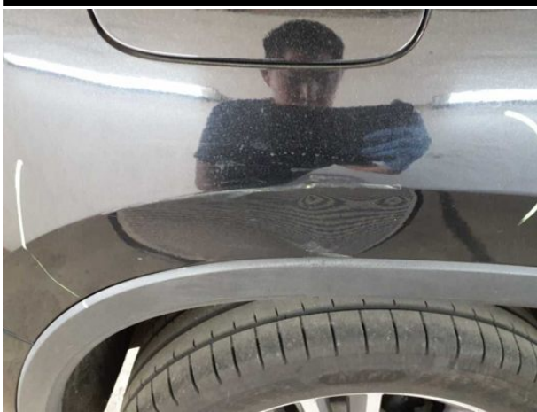
Damage #14: Side panel - rear right side: Side panel - Dent / paintcoat damage - Repair and paint
