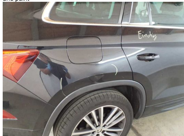
Damage #14: Side panel - rear right side: Side panel - Dent / paintcoat damage - Repair and paint
