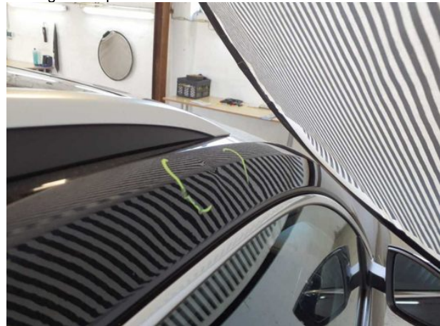
Damage #12: Roof: Roof rail - right side - dent(s) - Repair and paint
