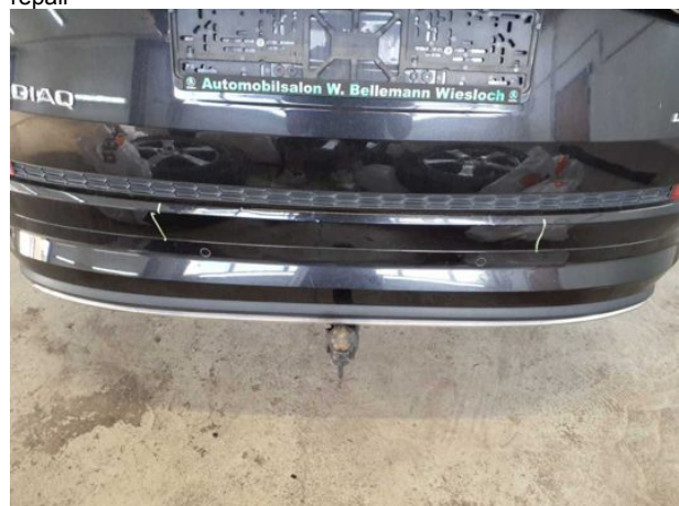
Damage #8: Rear bumper: Rear bumper - Scratched - Smart repair
