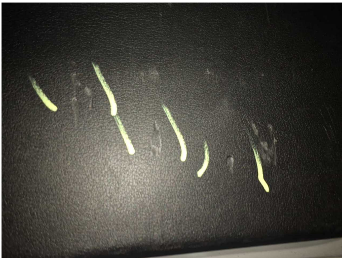
Damage 4: Trim / covers: Boot lid - interior trim - Scratch(es) - Replace
