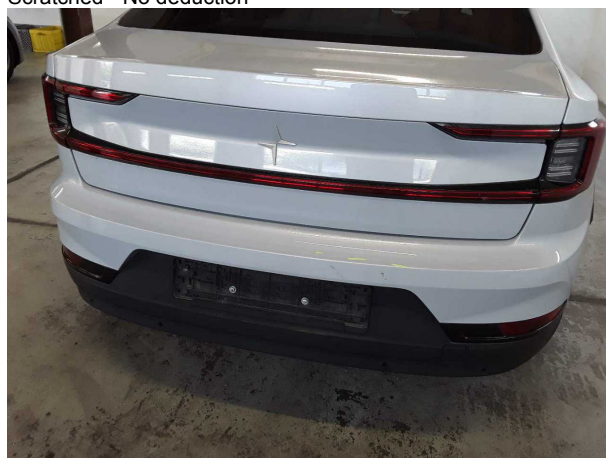
Damage #5: Rear bumper: Rear bumper - Scratch(es) - Covered area - No deduction
