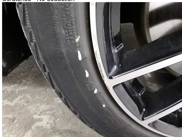
Damage #3: Wheel / tyres: Alloy rim - front right side - Scratched - No deduction
