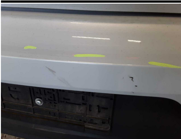
Damage #5: Rear bumper: Rear bumper - Scratch(es) - Cover / polish
