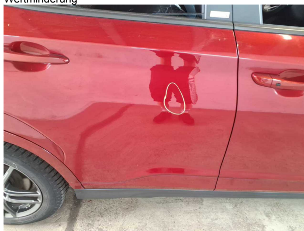
Beschädigung #4: Tür hinten rechts: Tür - Delle / Lackschaden - Smart Repair
