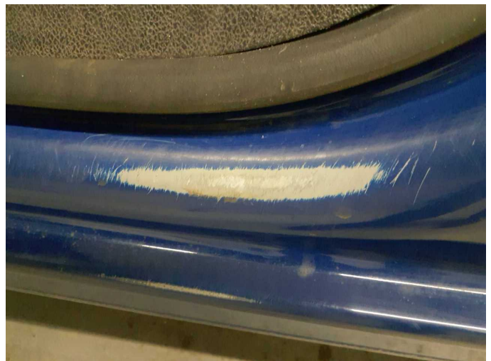
Damage 7: Sill - left side: Sill - Paint defect - Paint
