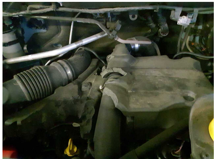
Damage 5: Cab: Insulation lining - Damage caused by marten / rodent - Replace
