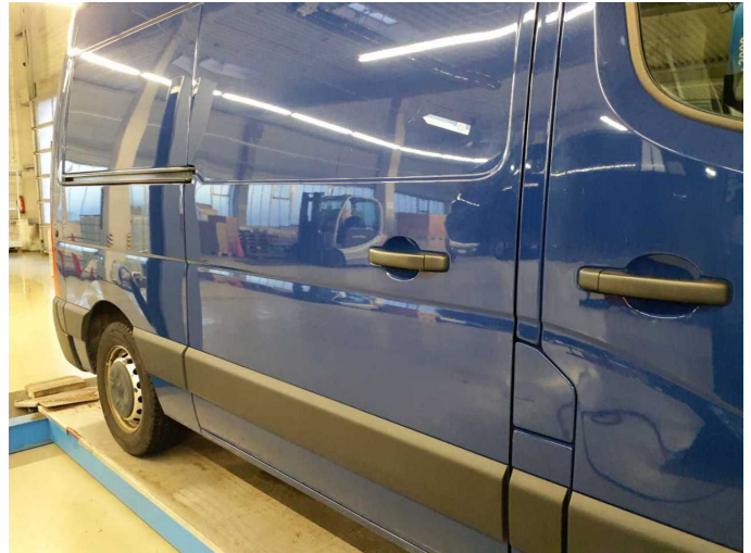
Damage 8: Sliding door, right: Sliding door - Dent / paintcoat damage - Repair and paint
