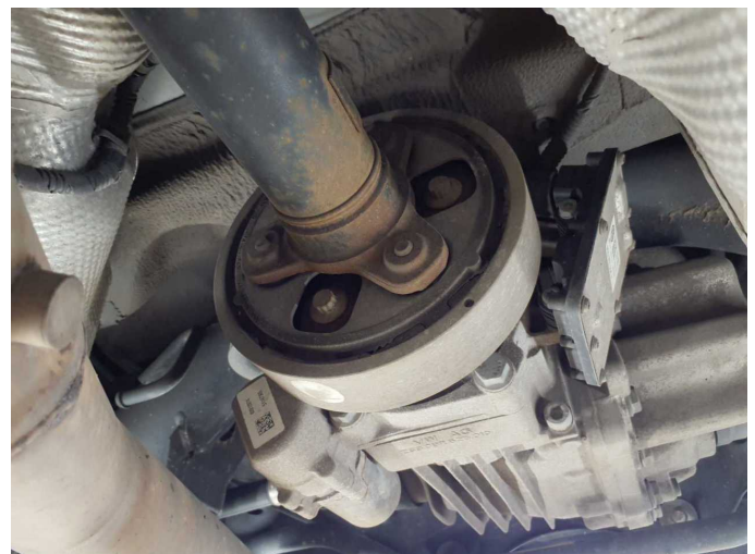
Damage 3: Drive train: Drive train (Harddiscs) - Porous / cracked - Replace
