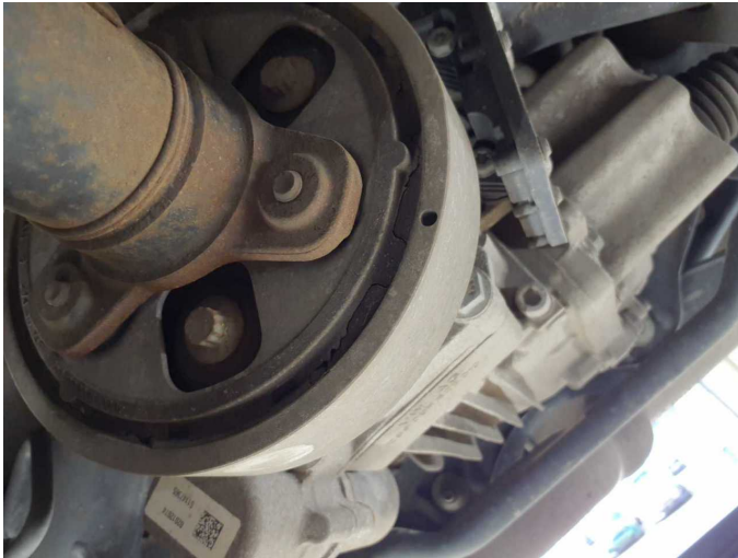
Damage 3: Drive train: Drive train (Harddachscheibe) - Porous / cracked - Replace
