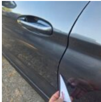
Damage Type Door-edge chipped
