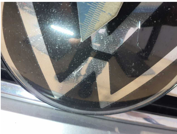
Damage 6: Front structure: Emblem - Stone chips - Replace
