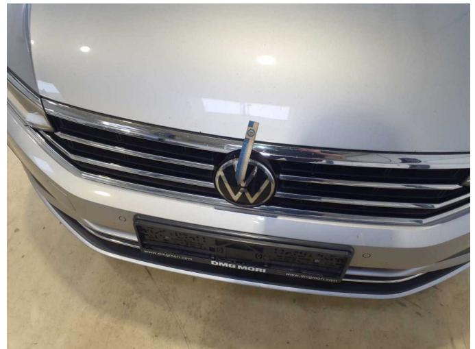
Damage 6: Front structure: Emblem - Stone chips - Replace
