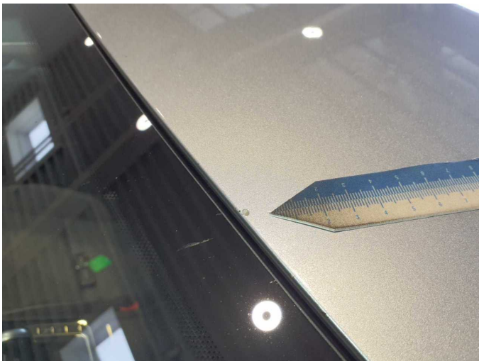
Damage 5: Roof: Roof - Stone chips - Smart repair
