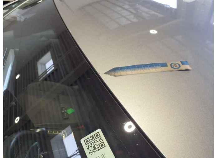
Damage 5: Roof: Roof - Stone chips - Smart repair
