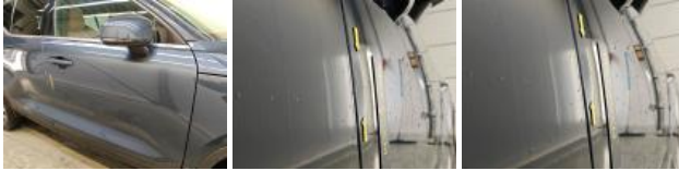
Door FR, Dent(s), Repair and paint (complete)
