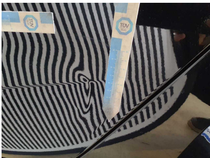
Damage 6: Door - rear left side: Door - Deformed - Repair and paint
