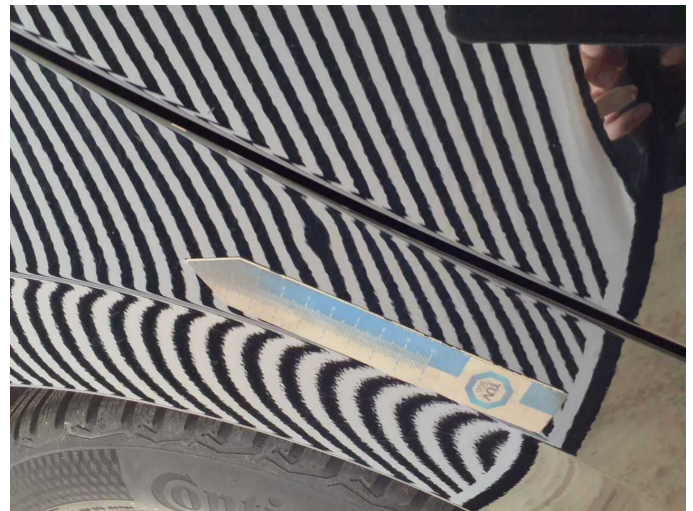
Wear and tear 3: Side panel - rear right side: Side panel - dent(s) - No deduction
