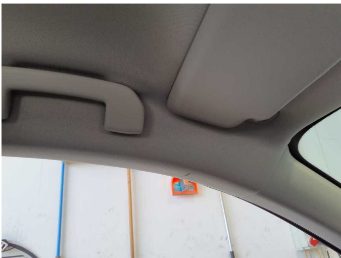
Damage 1: Trim / covers: Roof lining - Scratch(es) - Smart repair
