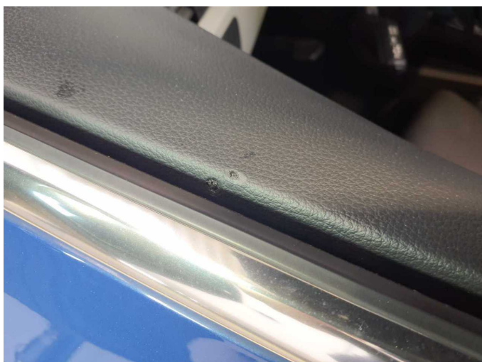
Damage 13: Trim / covers: Door trim - front left side - Burn hole (cigarettes) - Replace
