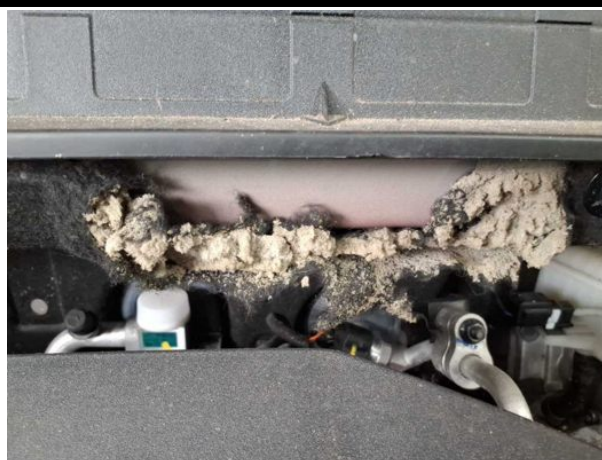
Damage #4: Cab: Insulation lining - Damage caused by marten / rodent - Replace
