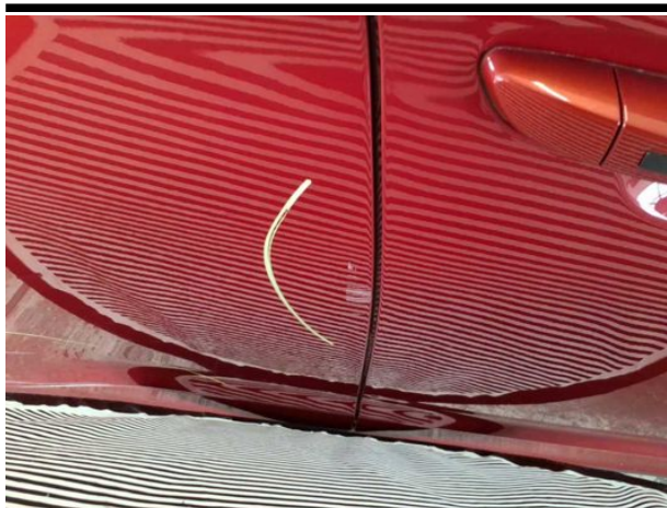
Damage #10: Door - rear right side: Door - Dent / paintcoat dama... - Repair and paint
