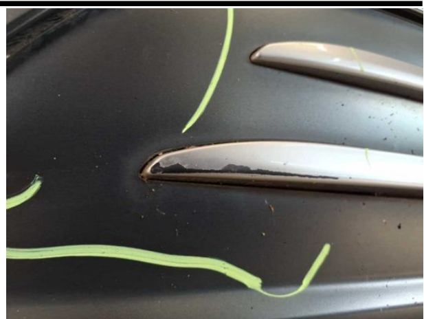
Damage #8: Rear bumper: Spoiler - Scratched - Replace
