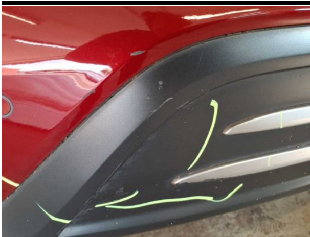
Damage #8: Rear bumper: Spoiler - Scratched - Replace
