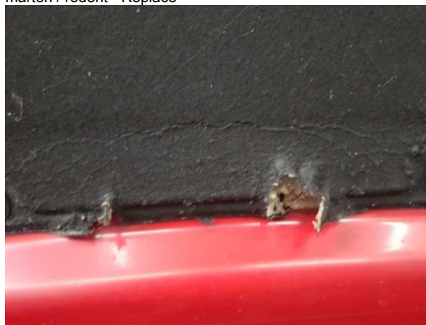
Damage #5: Bonnet: Insulation lining - Damage caused by marten / rodent - Replace
