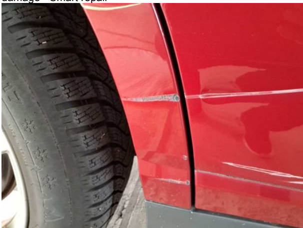
Damage #7: Side panel - rear right side: Wheel arch - Scratched - Replace
