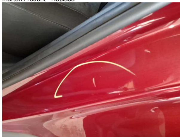
Damage #6: Side panel - rear left side: Sill - Dent / paintcoat damage - Smart repair
