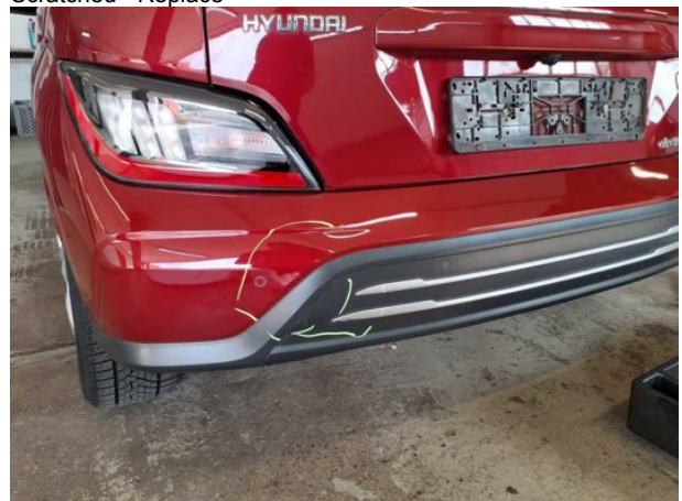
Damage #8: Rear bumper: Spoiler - Scratched - Replace
