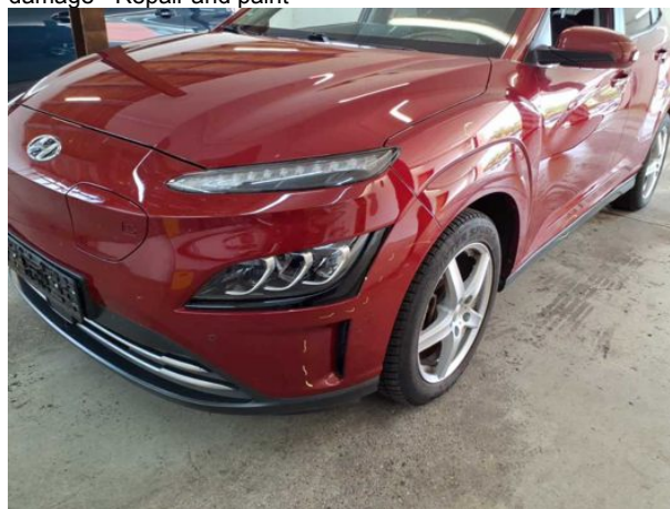
Damage #11: Front bumper: Front bumper - Scratched - Rep... and paint
