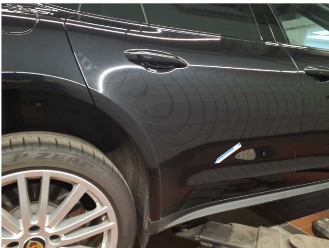
Damage 9: Door - rear right side: Door (Rostunterwandert+ Steinschläge) - Corrosion - Repair and paint
