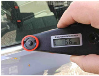
Paint thickness Door RR
