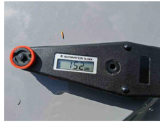
Paint thickness Wing FL
