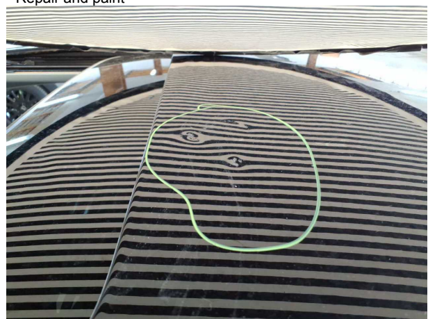
Damage #9: Roof: Roof - Dent / paintcoat damage - Repair a... paint
