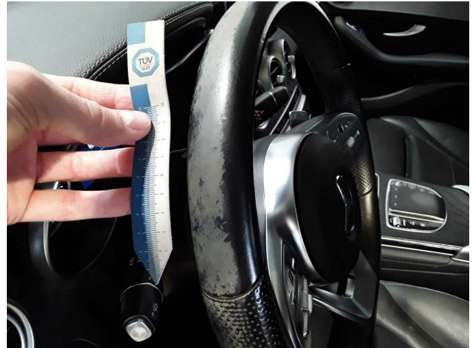
Damage 2: Steering system: Steering wheel - Worn - Smart repair
