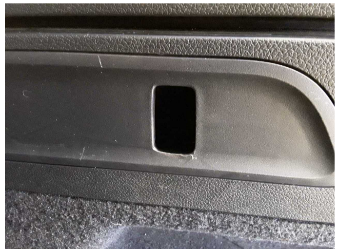
Damage 1: Trim / covers: Cargo area - lining - right side (Taster Sitzentriegelung reingedrückt) - Differs from the original configuration - Un- / install
