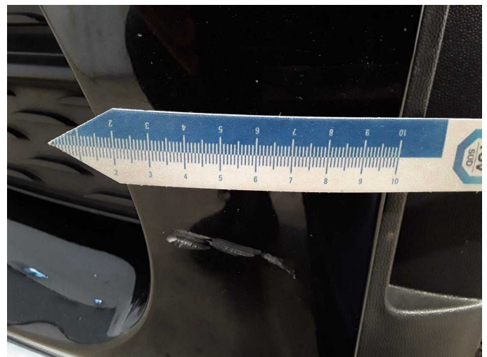
Damage 4: Front bumper: Front bumper - Scratch(es) - Paint
