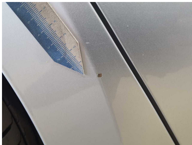
Damage 6: Side panel - rear right side: Side panel - Corrosion - Repair and paint
