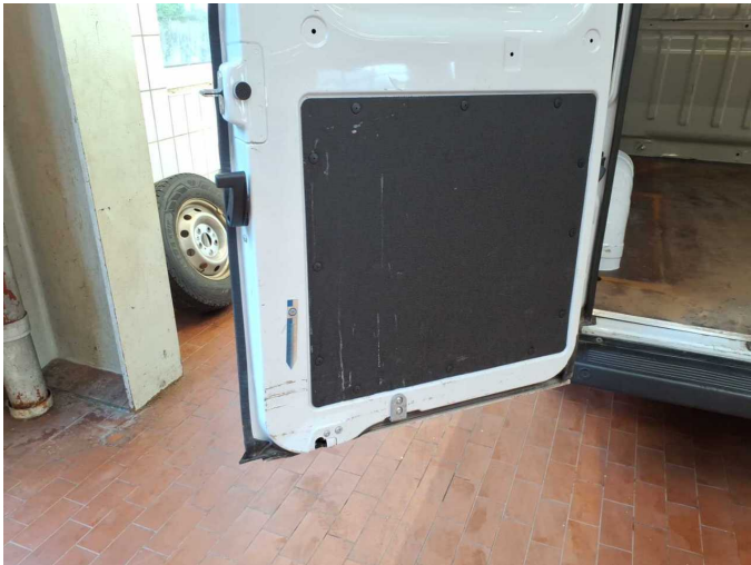
Damage 8: Boot lid / rear door: Rear door - left side (Innen) - Dent / paintcoat damage - Loss in value
