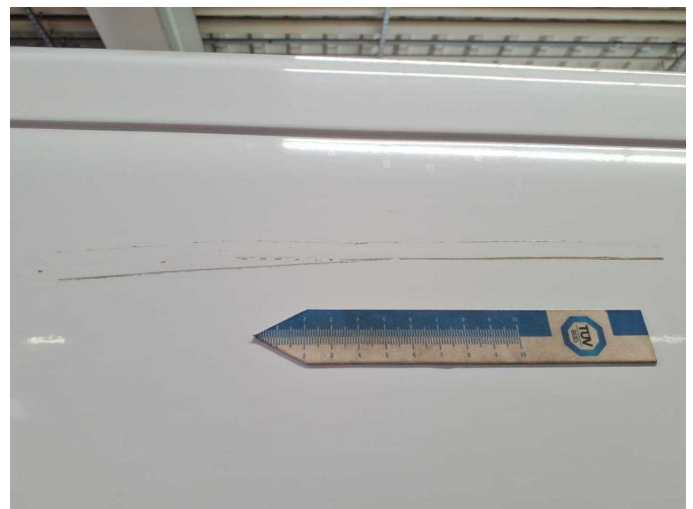
Damage 12: Side panel - rear right side: Side panel (Oben + Delle) - Scratched - Repair and paint
