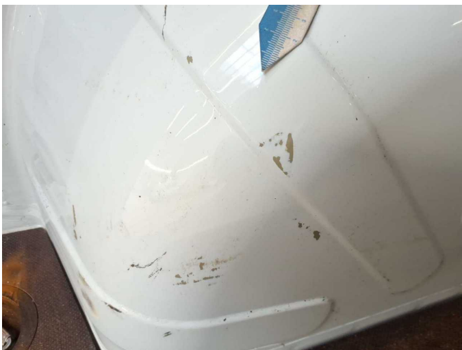
Wear and tear 4: Body: Wheel well - rear left side (Innen) - Scratch(es) - No deduction
