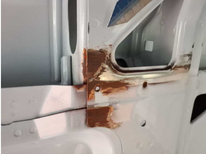
Damage 9: Side panel - rear left side: Side panel (Innen) - Corrosion - Smart repair
