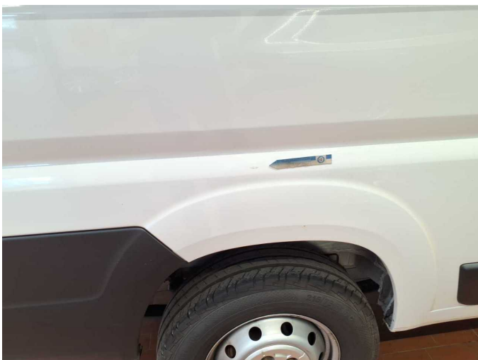
Damage 6: Side panel - rear right side: Side panel (unten) - Scratch(es) - Smart repair
