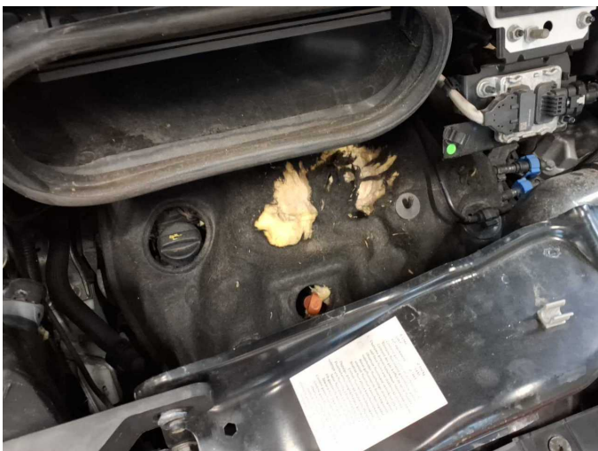
Damage 2: Engine: Engine cover (Isolierung Motor) - Damage caused by marten / rodent - Replace
