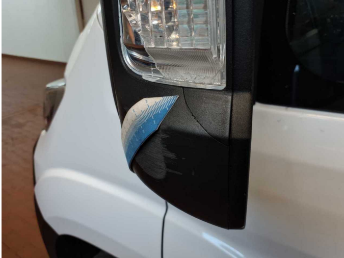
Damage 11: Wing mirror - left side: Mirror housing (Spiegelblinker li. gebrochen) - Broken / torn - Replace
