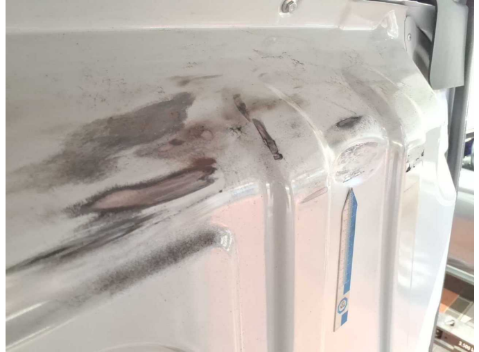
Damage 3: Body: Partition wall - Dent / paintcoat damage - Loss in value
