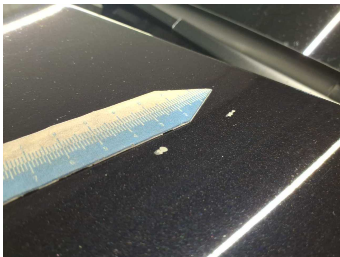
Damage 10: Bonnet: Bonnet - Stone chips - Paint
