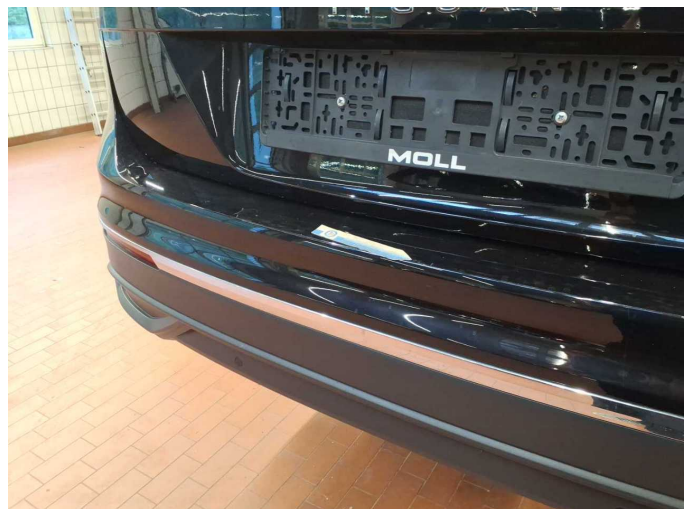
Damage 9: Rear bumper: Rear bumper - Scratch(es) - Paint
