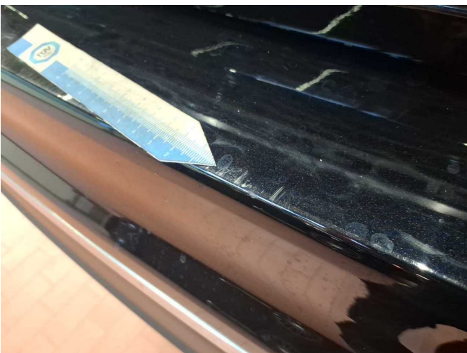
Damage 9: Rear bumper: Rear bumper - Scratch(es) - Paint
