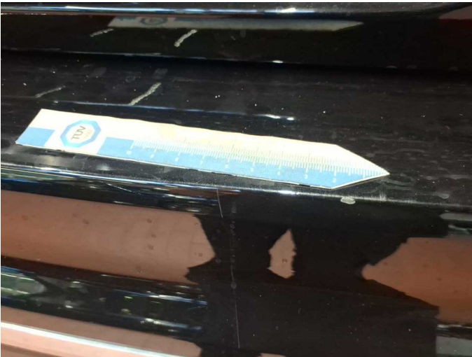
Damage 9: Rear bumper: Rear bumper - Scratch(es) - Paint
