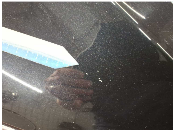
Damage 10: Bonnet: Bonnet - Stone chips - Paint
