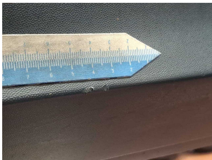
Wear and tear 1: Door - front left side: Brightware - lower - Scratch(es) - No deduction
