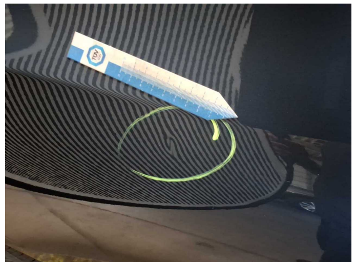
Damage 1: Door - rear right side: Door - dent(s) - Smooth repair work
