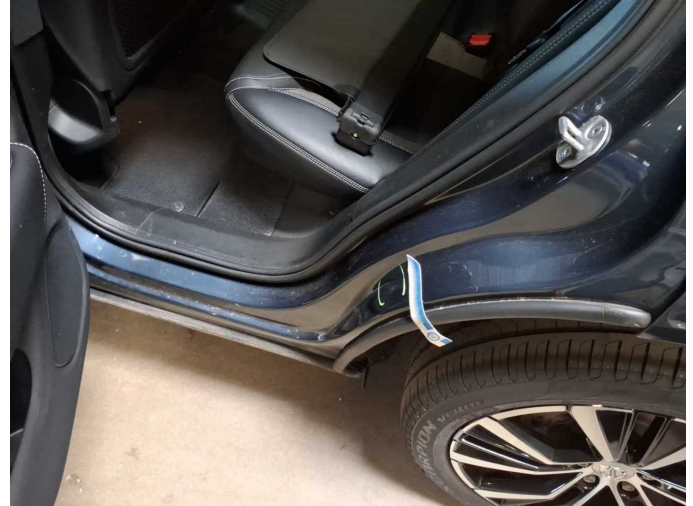
Damage 2: Side panel - rear left side: Sill - dent(s) - Smooth repair work
