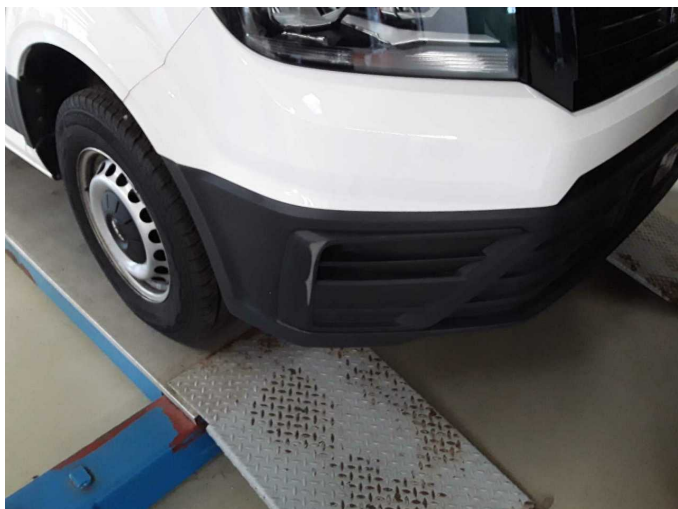
Damage 2: Front bumper: Front bumper - Scratch(es) - Replace
