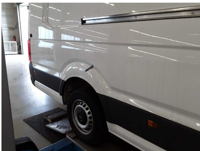
Damage 6: Side panel - rear right side: Side panel (Orangenhaut / wolkig / wellig / Schleifspuren) - Unprofessionally repaired - Repair and paint
