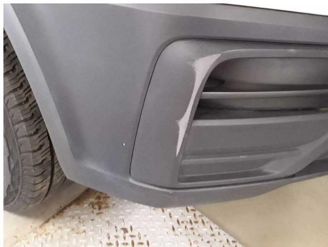
Damage 2: Front bumper: Front bumper - Scratch(es) - Replace
