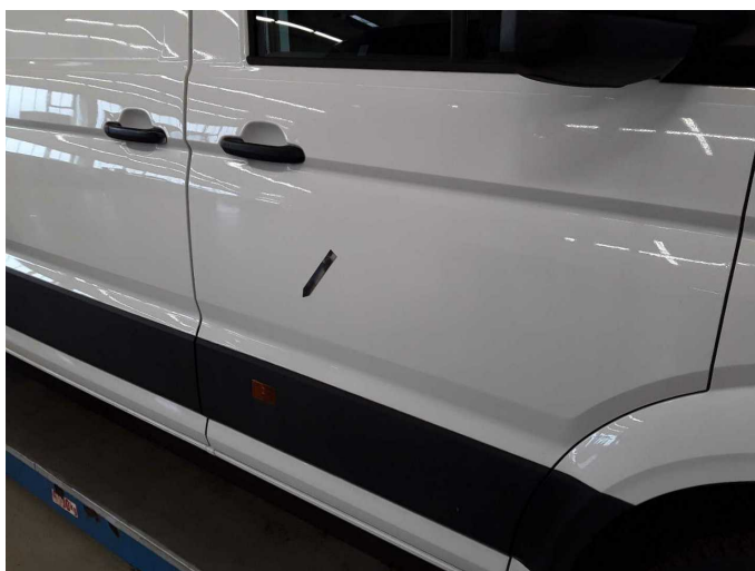
Damage 5: Door - front right side: Door (wellig) - Unprofessionally repaired - Repair and paint
