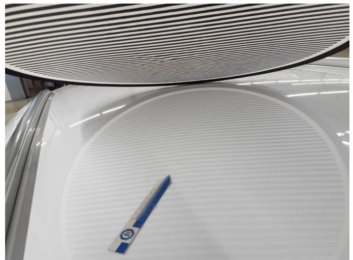
Damage 3: Roof: Roof - dent(s) - Smart repair
