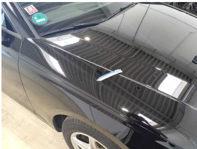
Damage 10: Bonnet: Bonnet - Scratch(es) - Paint
