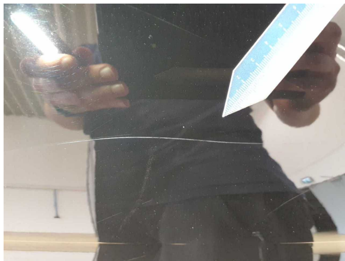
Damage 10: Bonnet: Bonnet - Scratch(es) - Paint
