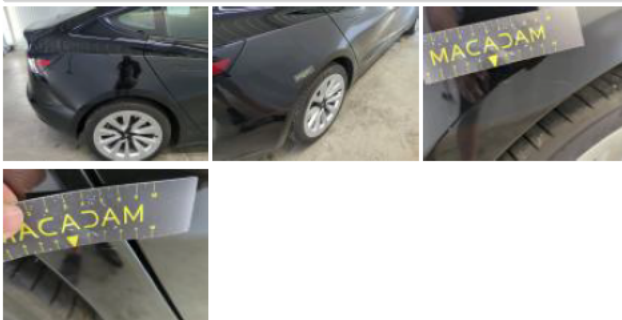
Door RR, Scratch(es), Repair and paint (complete)
