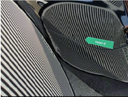
Kotflügel / Hinten Links / Delle
