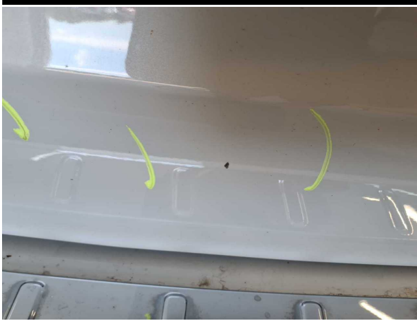
Damage #3: Boot lid / rear door: Boot lid - Dent / paintcoat damage - Repair and paint
