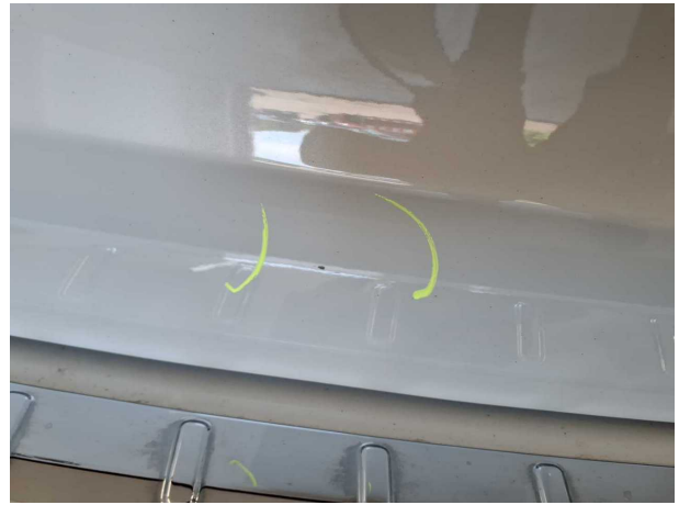
Damage #3: Boot lid / rear door: Boot lid - Dent / paintcoat damage - Repair and paint
