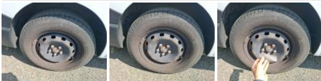
Wheel cover FR, Missing, Replace
