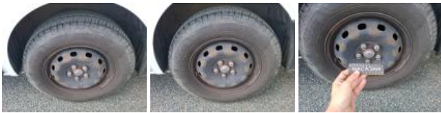
Steel rim RL, Deformed / Strained, Replace
