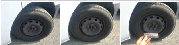
Side wall RL, Dent(s), Acceptable
