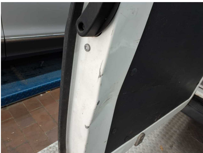
Damage 5: Boot lid / rear door: Rear door - left side - Dent / paintcoat damage - Replace
