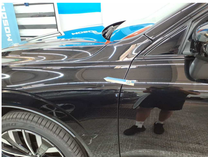
Damage 2: Mudguard - left side: Mudguard - left side (Polieren) - Scratch(es) - Smart repair
