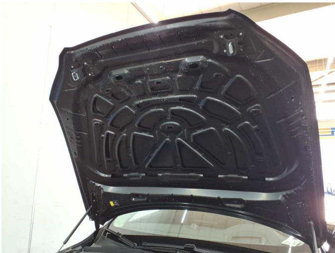
Damage 7: Bonnet: Insulation lining - Missing - Replace
