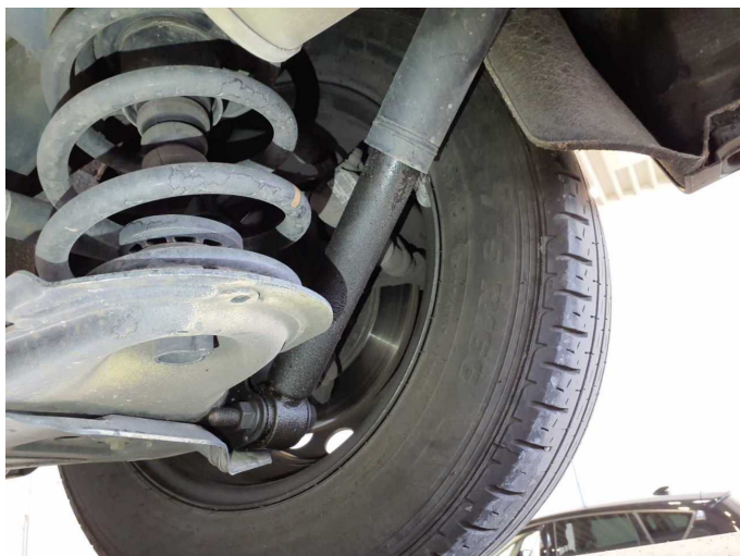
Damage 8: Rear axle: Shock absorber - right side - Leaking - Replace
