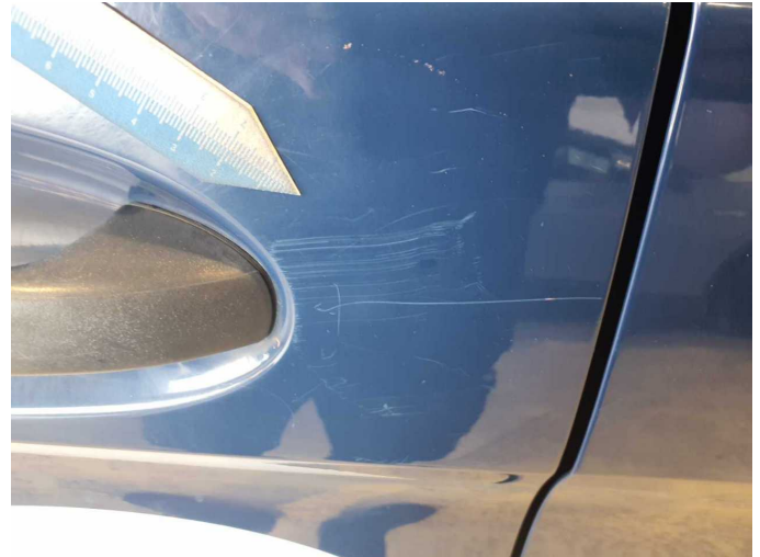
Damage 11: Sliding door, right: Sliding door - Scratch(es) - Paint
