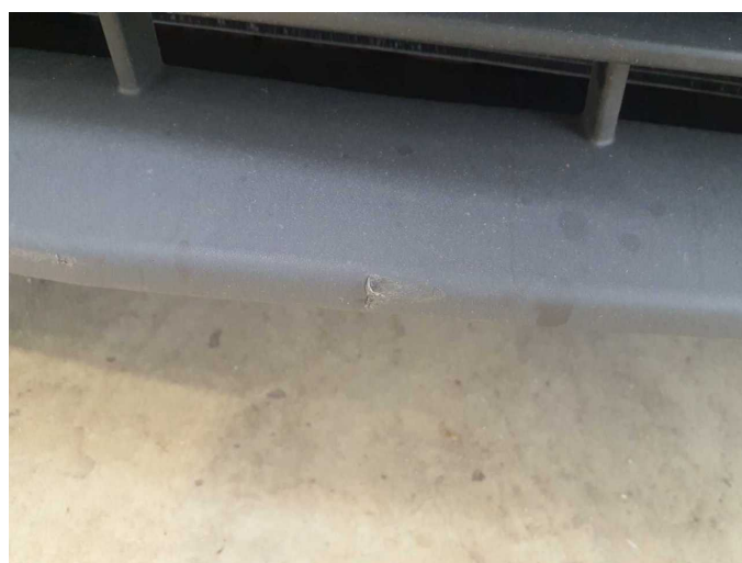
Damage 4: Front bumper: Front bumper - Scratch(es) - Loss in value
